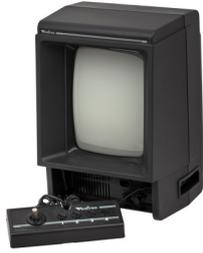
The Vectrex is the one and only games console that employs vector scan rather than raster scan technology to generate images. This means that the game graphics are represented by line drawings rather than bitmaps. As such the graphics are very distinct. The appearance of the sharp white lines on a black background make the Vectrex look as though it comes from another world.
